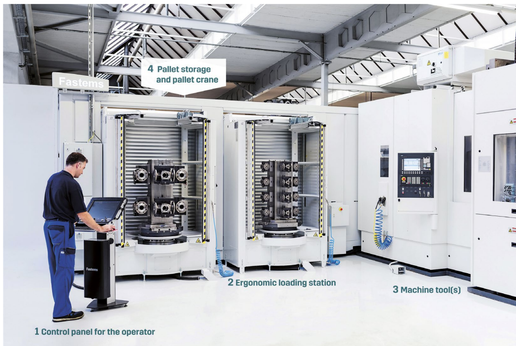
10 Linear pallet automation system consists of a production control panel, ergonomic loading station, machine tool(s), pallet storage and a crane that moves pallets in the system. This example is Fastems' Flexible Pallet Container FPC.
