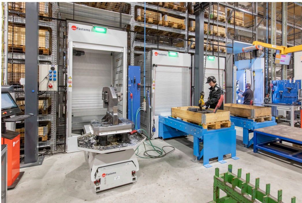
9 Ergonomic loading stations for raw materials and machining pallets enable less consuming work for operators.
